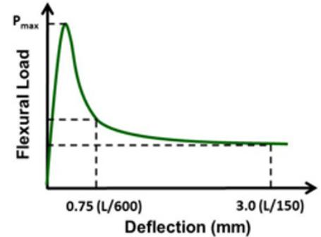
Schematics of a typical C1609 test result
