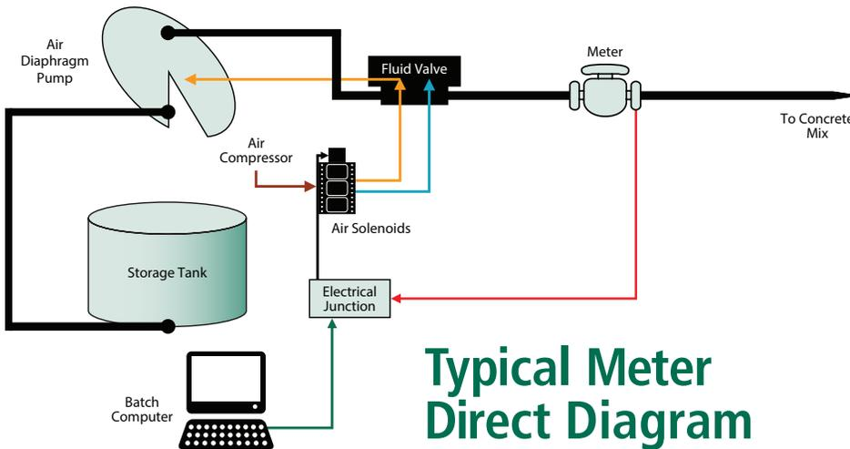
**Typical Meter Direct Diagram**
