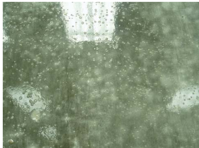
Bubbles can form in a sealer when it is applied too thick; it is recommended to apply sealer in two thin layers.
