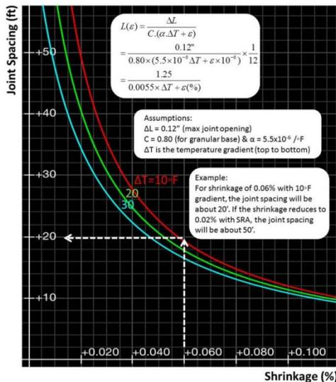
This graph shows typical recommended joint spacing criteria (Darter and Barenberg, 1977) and has been used in FHWA reports and multiple publications.
