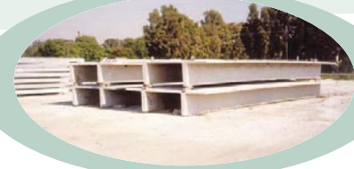
Plastol 5000 superplasticizer and Eucon MSA microsilica are used to achieve very high flexural and compressive strengths
